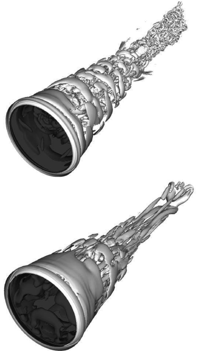
Fig. 9 Instantaneous isocontours of Q = 0.1 for DNS (top) and FSM calculation on fine grid, k_{\max} = 32 and \beta = 1 \times 10^{-3} (bottom), perspective view from inflow towards outflow; Re_D = 6 \times 10^4 , M = 2.46 .
